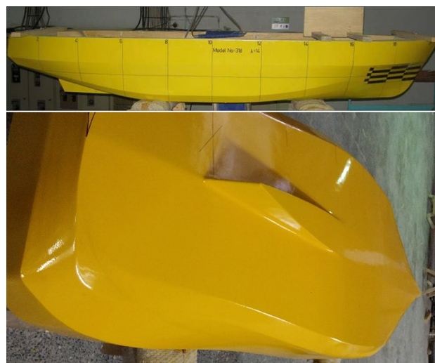
Fig. 15 Side view of the original Model M318-0 (above), DWL-optimized model M318-1 (below)
