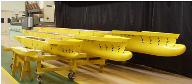
Fig. 1 Models of the 8,600-TEU container carrier
