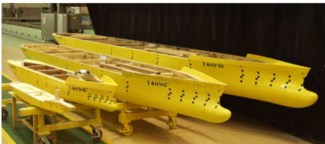
Fig. 2 Models of the 155,000- m^3 liquefied natural gas (LNG) carrier
