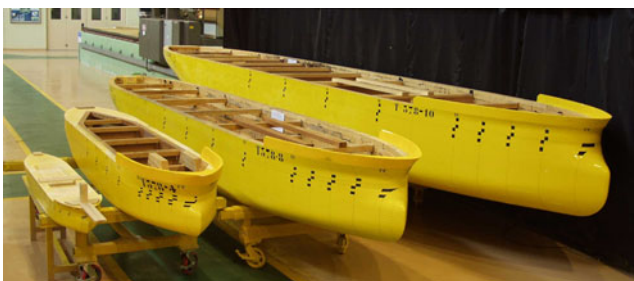
Fig. 3 Models of the 317,000-TDW very large crude carrier (VLCC)
