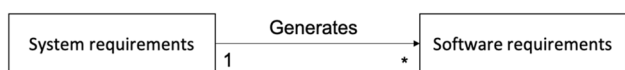
Fig. 3 An example of a simple TIM with one trace link type (generates) which connects system requirements to software requirements
