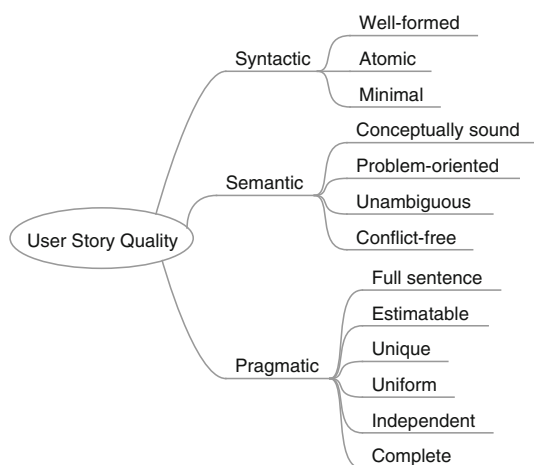
Fig. 2 Quality User Story framework that defines 13 criteria for user story quality: overview
