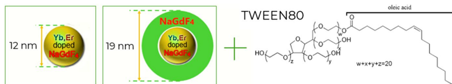
Fig. 2 Schematic presentation of two kinds of UCNP both functionalized with surfactant TWEEN80: 12 nm NaGdF 4 :Yb, Er core and 19 nm NaGdF 4 :Yb, Er@NaGdF 4 core-shell, where the 12 nm core was additionally coated with 7 nm of NaGdF 4 optical inert layer
