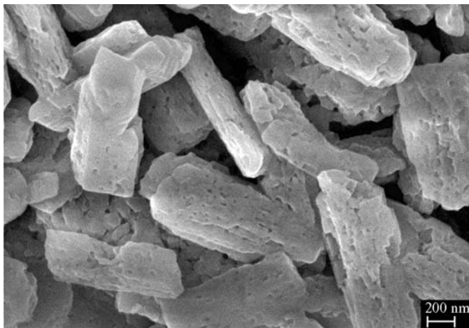
Fig. 9. SEM micrograph of the alumina-pinned \text{Ga}_2\text{O}_3 crystallites after annealing at 1200 °C.
