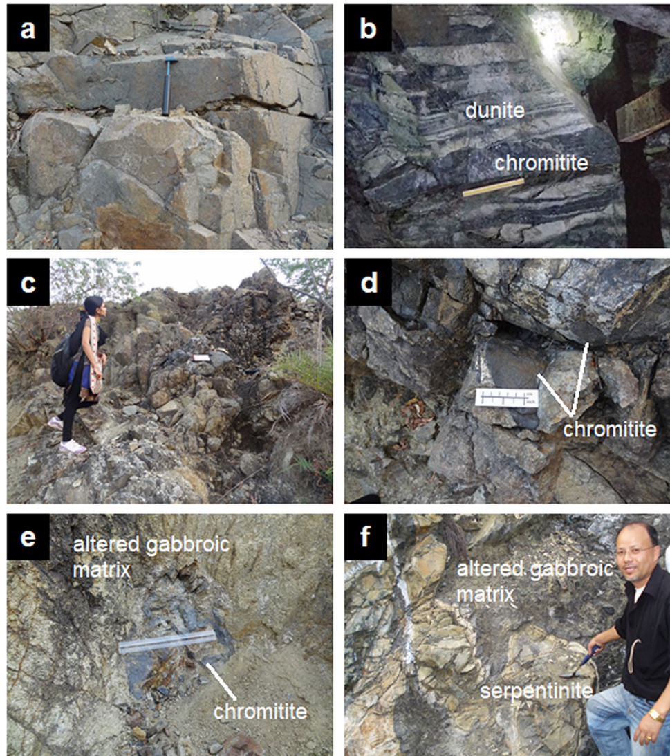
Fig. 2 a Gabbro-anorthosite rock near the opencast Bangur mining area; b Alternate layers/bands of dunite and chromitite that are faulted (underground mines at +30 mRL), the scale is 30 cm; c Field photograph showing the brecciated zone on the surface; d Sub-rounded chromitite clasts embedded within the brecciated ultramafic rocks; e A chromitite boulder within highly altered ultramafics near top bench of Bangur opencast mine; the scale is 30 cm; f both dunite boulders and gabbro matrix have been severely altered to serpentinite and chloritite respectively near Nuasahi in the Bangur gabbro breccia apophysis
