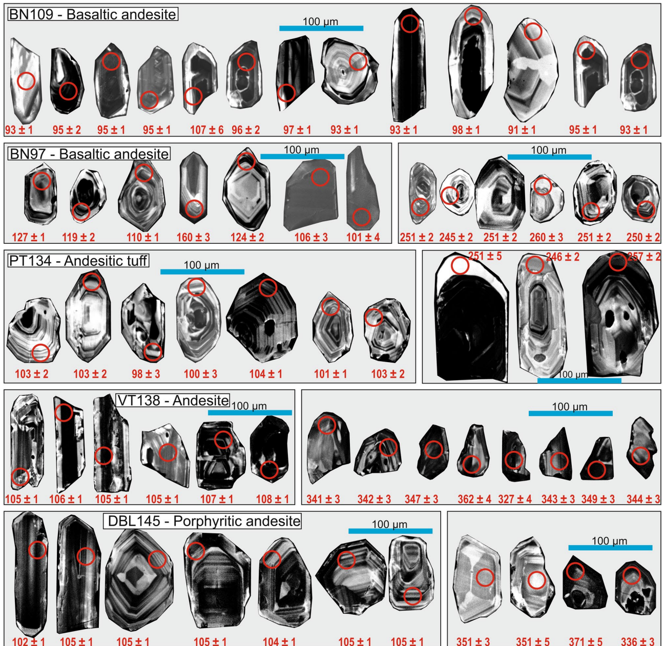
Fig. 9 Cathodoluminescence (CL) images of representative zircon from volcanic rocks in the Bay Nui area (BN109 and BN97) and Dalat zone (PT134, VT138, and DBL145)
