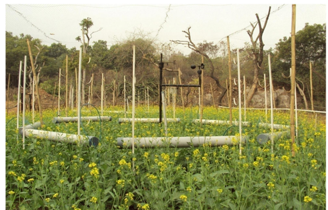
Fig. 1 Free air carbon dioxide enrichment (FACE) facility built on the campus of Jawaharlal Nehru University, New Delhi, India. Mustard ( Brassica ) plants were grown inside FACE rings maintained at elevated CO 2 (585 μmol mol -1 )
