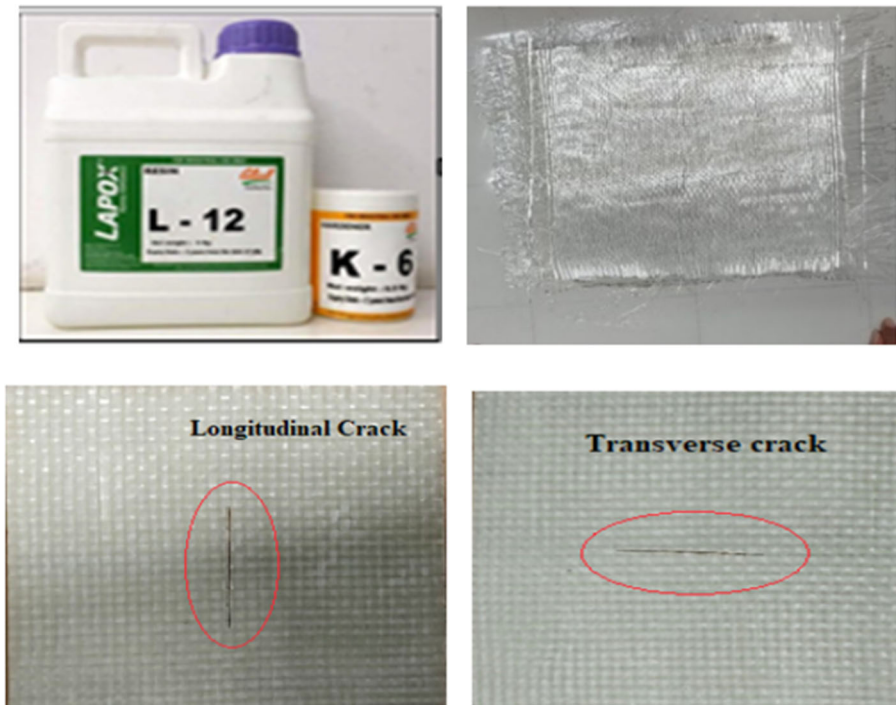
Fig. 3 Materials and fabricated laminated composites
