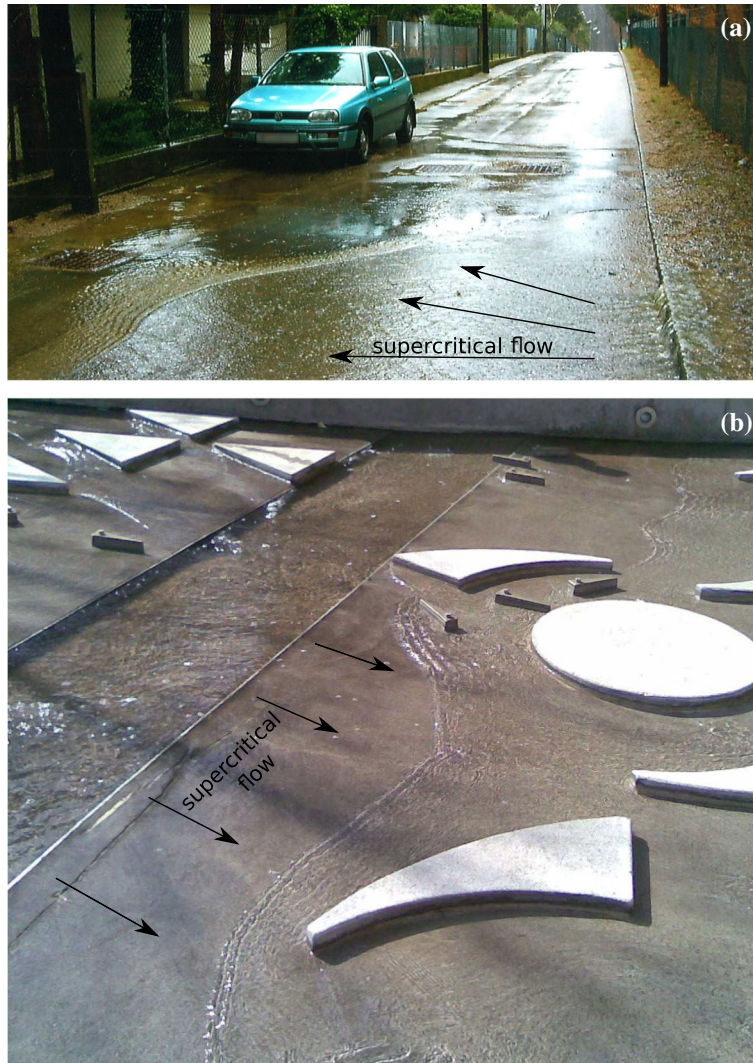
Fig. 1 a Observation of an undular hydraulic jump with concave front. Photograph taken by R. Kolda in Vienna, Austria on 7 March 2009. b Observation of an undular hydraulic jump with convex front. Photograph taken by H. Steinrück in Karlsruhe, Germany on 24 March 2010
