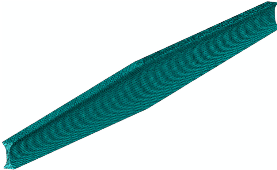
Fig. 6 Exemplary FEM model of the beam with linearly varying depth for numerical studies
