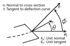
Fig. 1 Diagram of relevant angles and vectors
