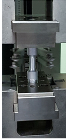
Fig. 1 The sample subjected to the cyclic tension–compression test
