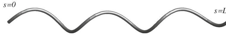
Fig. 1 Equilibrium configuration of a nonlocal rod with the end at s = 0 clamped and the end at s = L constrained to have the tangent parallel to the undeformed axial curve \mathcal{C}^u , subject at the end s = L to a force parallel to \mathcal{C}^u and a couple whose component parallel to \mathcal{C}^u is assigned. In dimensionless units the length of the rod is L = 360 , its circular cross section has diameter d = 4 , the force is F = 6.853 \times 10^{-4} , and the twisting moment is \alpha = -3.75 \times 10^{-2}
