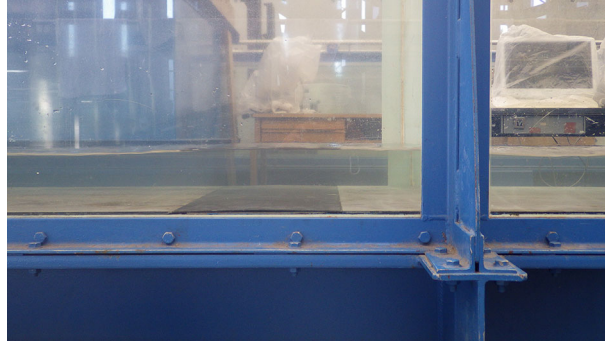
Fig. 5 Part of the test section. Light grey: plane steel plates. Dark grey: bump
