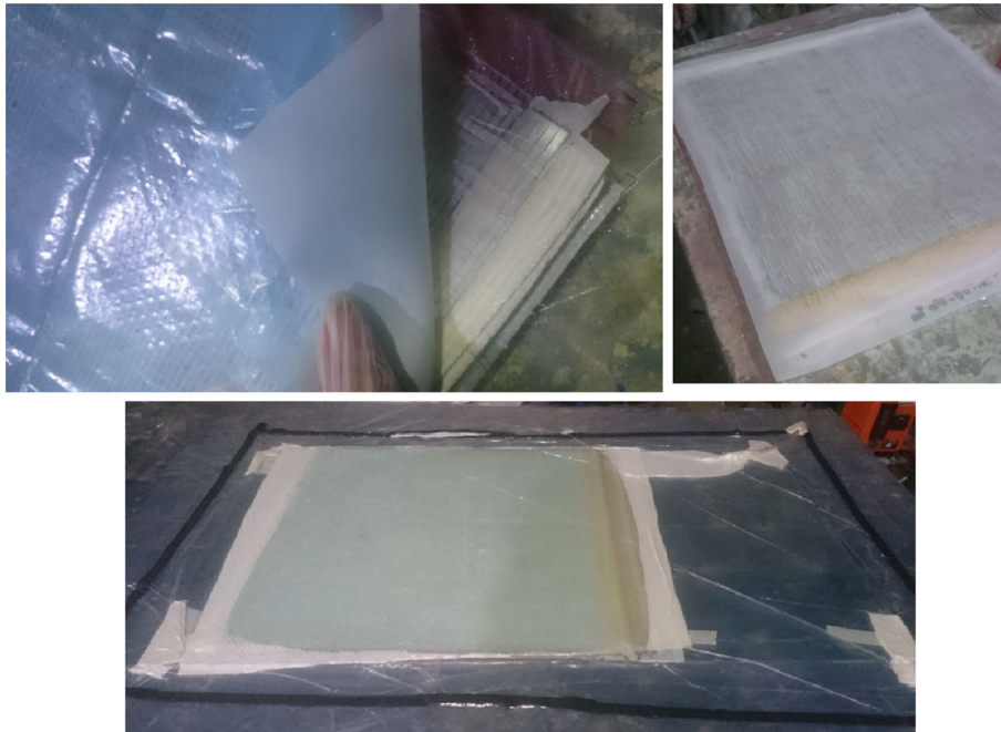
Fig. 4 Placing the Dacron textile and perforated film on the fibers and resin set
