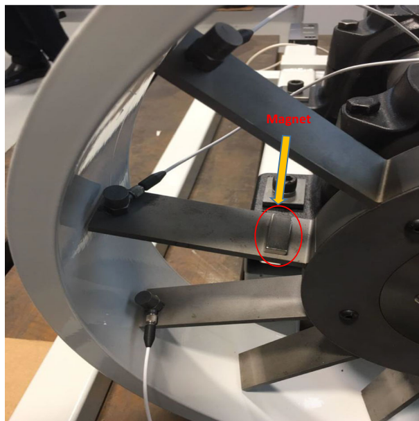
Fig. 13 a Impact hammer test setup, b front view of the setup
