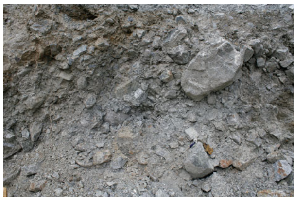
Fig. 1 Fragmented material in the deposits of the Val Pola landslide, northern Italy. Picture field about 1.5 \times 2 m
