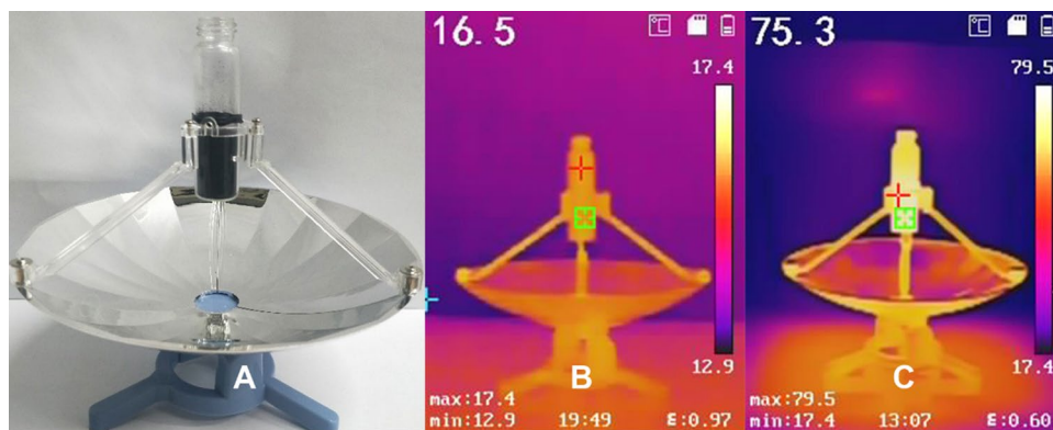
Fig. 10 Reaction set (A) for photothermal desorption of carbon dioxide. Infrared thermography of the set in the dark (B), or under simulated sunlight (C)
