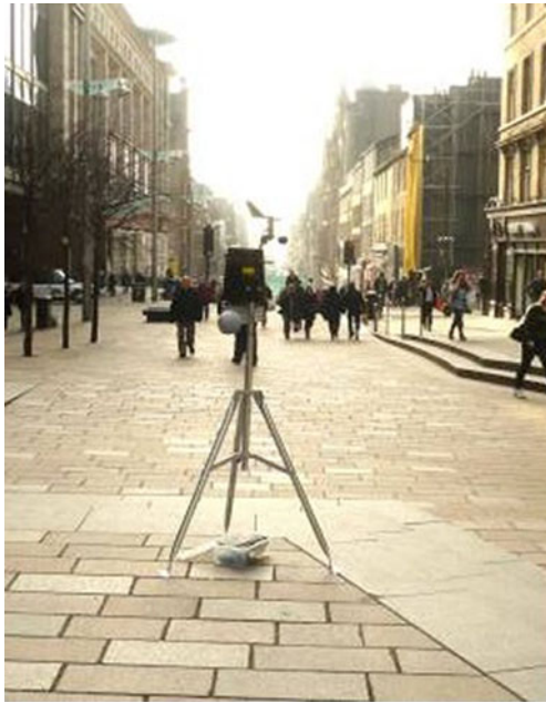
Fig. 2 'Mobile' weather station (Davis Vantage Pro2) with grey globe thermometer, at Point 1
