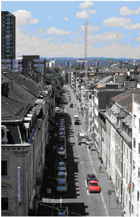
Fig. 2 The street canyon from above (Sperrstrasse). The tower reaches approximately 2.2 times the mean roof height of the urban surface (photography obtained from the internet page of the BUBBLE experiment)
