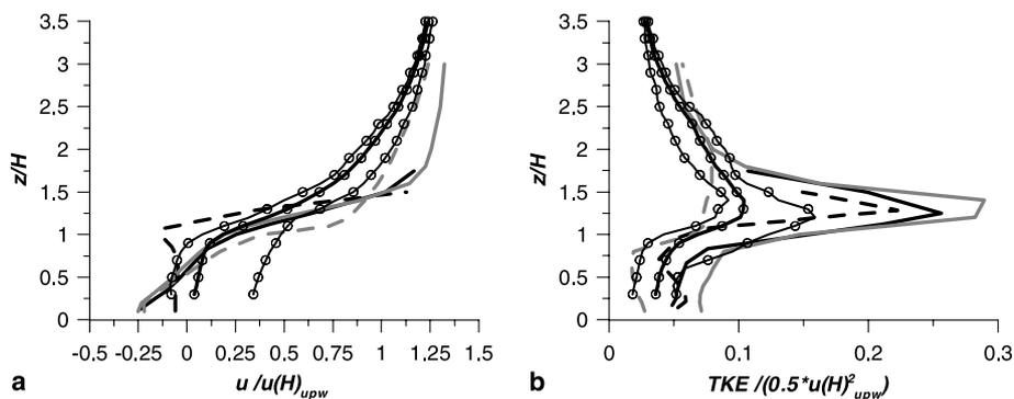
**Fig. 6.** Averaged profiles of the  $u$ -velocity component (a) and turbulence kinetic energy (b). Black lines: IC-UKA, solid for flat roofs and dashed for slanted upwind roof. Gray lines: IC-EPA, solid for first canyon and dashed for sixth canyon. Circles: RC-UKA (thick line – mean; thin lines – lowest/highest values)
