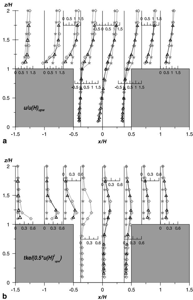
**Fig. 5.** Profiles of the  $u$ -velocity component (a) and TKE (b) in the central vertical plane of idealized street canyons. Triangles: IC-UKA,  $L = 120$  cm. Diamonds: IC-EPA, first canyon. Stars: IC-EPA, sixth canyon
