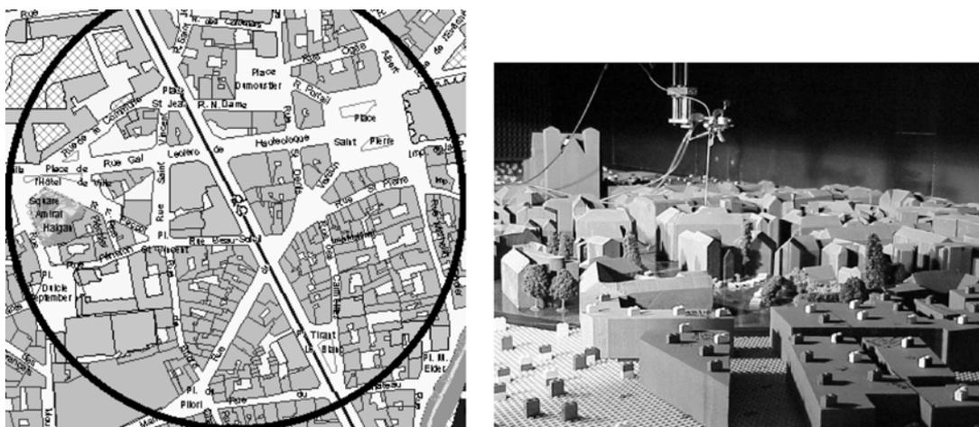
**Fig. 1.** Example of a complex urban street canyon situation: The left plot shows a street map with building contours for a central part of Nantes, France. The right picture shows a photo of a detailed wind-tunnel model in which the encircled area was reconstructed on the scale: 1:200 (Kastner-Klein and Rotach, 2004)
