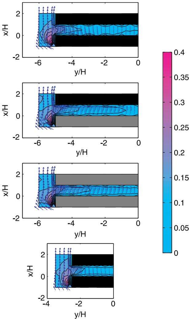
**Fig. 4.** Velocity in a horizontal plane at  $z/H=0.25$  of isolated street canyons with  $L/H=10$  and 5 for different roof configurations (due to symmetry only one half of the canyon is shown,  $y/H=0$  corresponds to the canyon centre). Buildings with flat roofs are plotted in black; buildings with pitched roofs are plotted in grey. The mean velocity field is shown by vectors, the colors refer to  $\sigma_u/u_0$
