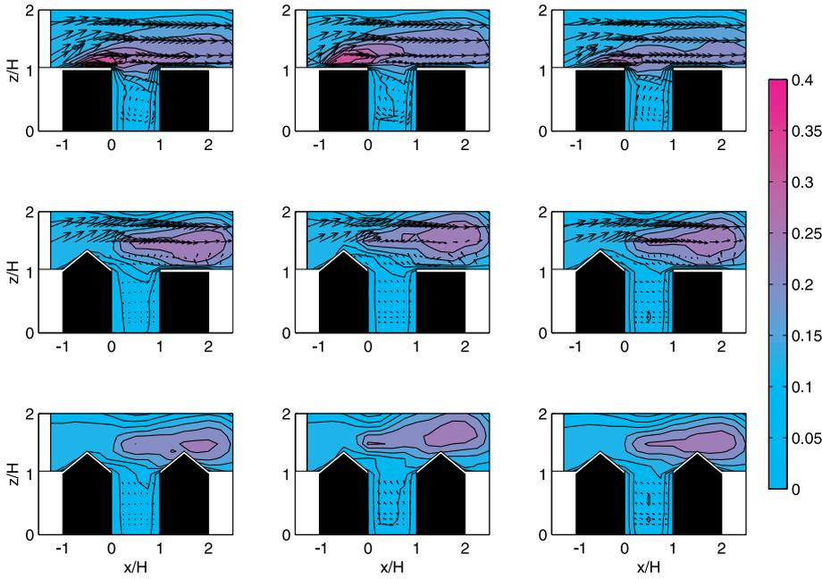
**Fig. 3.** Velocity in the central vertical plane of isolated street canyons with  $L/H = 15$  (left plots), 10 (middle plots) and 5 (right plots) for three different roof configurations. The mean velocity field is shown by vectors, the colors refer to  $\sigma_u/u_0$
