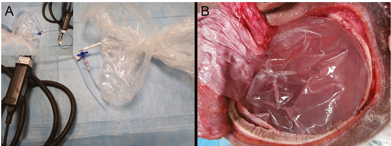
Fig. 2 Experimental measurement system. A Plastic bag containing saline solution, three-way connector, and pressure transducer; B measurement system placed inside the specimen's skull
