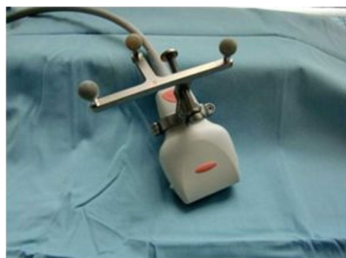
Fig. 1 Toshiba PLT-704SBT tracked linear ultrasound probe for integration into the neuronavigation system
