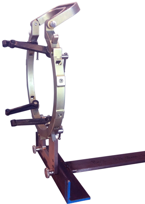
Fig. 1 This low profile frame holder is fixed to the operating table. The patient's head is fixed to the frame and the CT scan performed. With the frame attached to the table the vertical position can be obtained compensating for the fixed position of the gantry. The patient position will not be changed until after the biopsy
