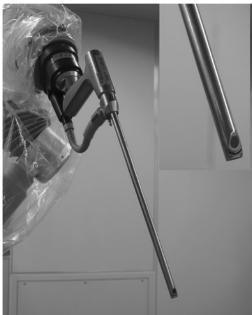
Fig. 1 A photograph showing the bayonet-shaped configuration of the endoscope. Close-up view of the tip with 70-degree side-viewing lens is demonstrated in the inset
