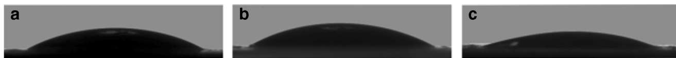
Fig. 2 Static water contact angles of water droplets on GO-CNF (a), PDA/GO-CNF (b), and Apt-Cys/PDA/GO-CNF (c) coated silicon wafer surfaces
