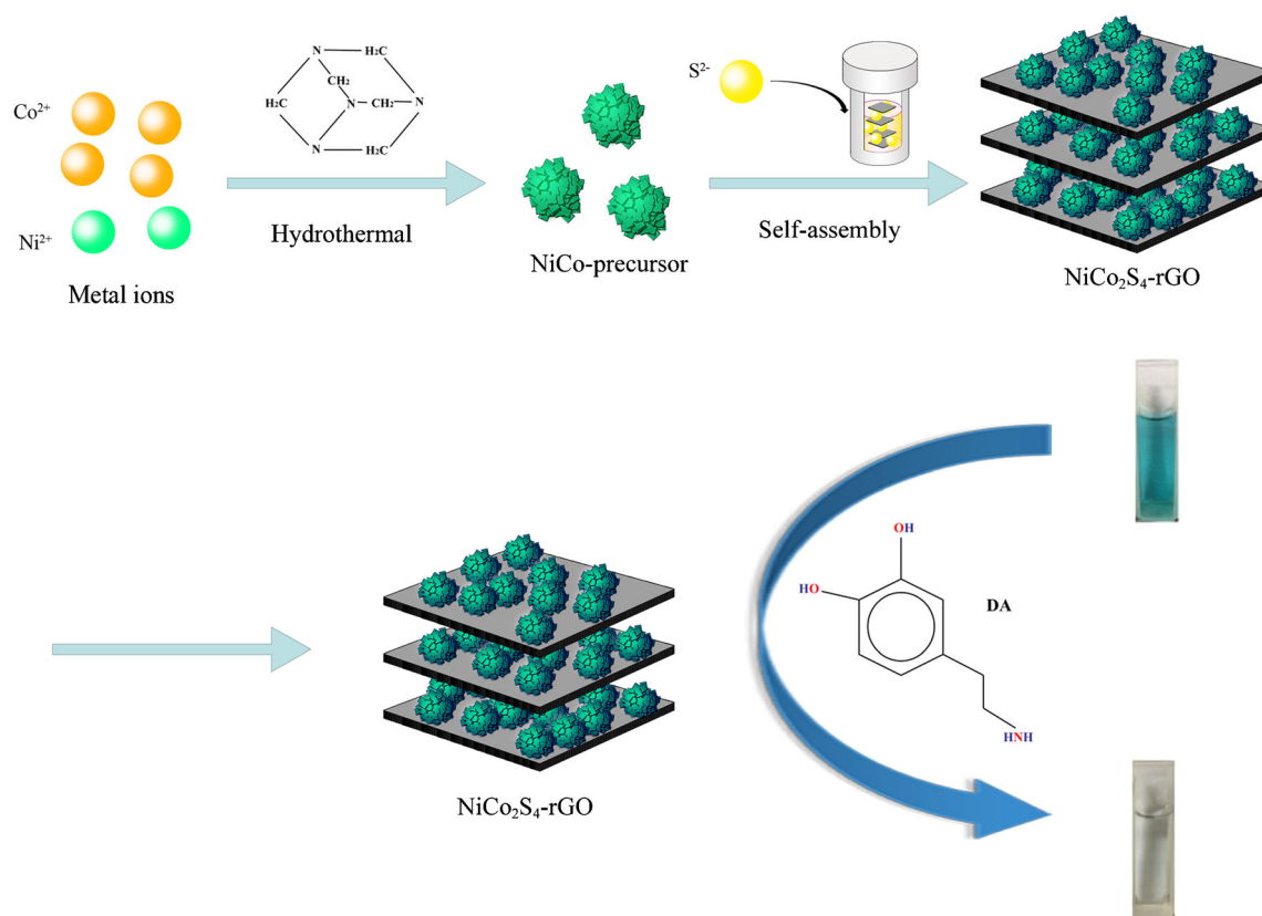
Scheme 1 Schematic diagram of the fabrication procedure for NiCo 2 S 4 -rGO composites and the colorimetric assay
