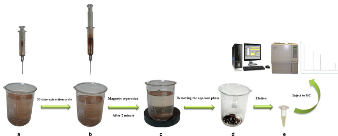
Fig. 2 Schematic representation of AA-d \mu -SPE. a 100 mL sample solution and 15 mg of adsorbents. b Suction and injection of solution using glass syringe was caused to increase of interaction between
