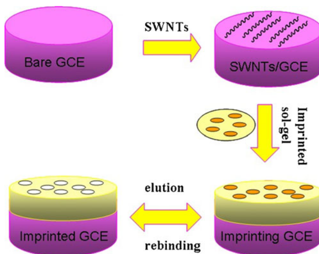
Scheme 1 The preparation of the MIP/sol-gel/SWNTs/GCE
