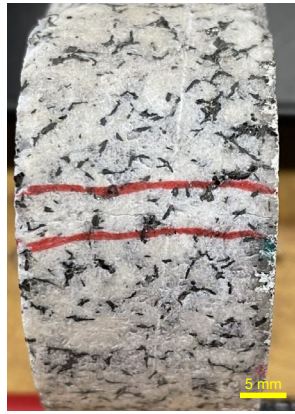
Fig. 15 Macrocrack trace, between the two red lines, at the circumferential surface of sample 25-S2 (Colour figure online)
