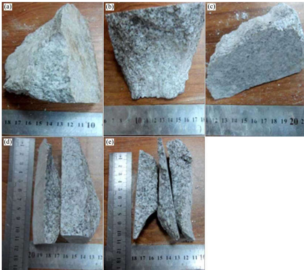
Fig. 2 Failure mode evolution process of granite specimens under different \sigma_2 (MPa): a \sigma_2=0 , b \sigma_2=10 , c \sigma_2=20 , d \sigma_2=30 , e \sigma_2=40 , after (Du et al. 2015)
