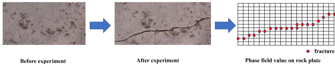
Fig. 15 The phase-field value on rock plate from the physical experiment. Random natural holes in the rock will affect the propagation of the artificial fracture. By using image technology, the phase-field
