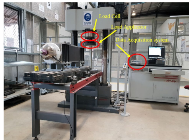
Fig. 1 Outline of SANS Machine used for double shear testing
