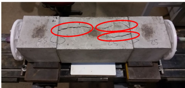
Fig. 6 Severe damage resulting from a weak concrete matrix
