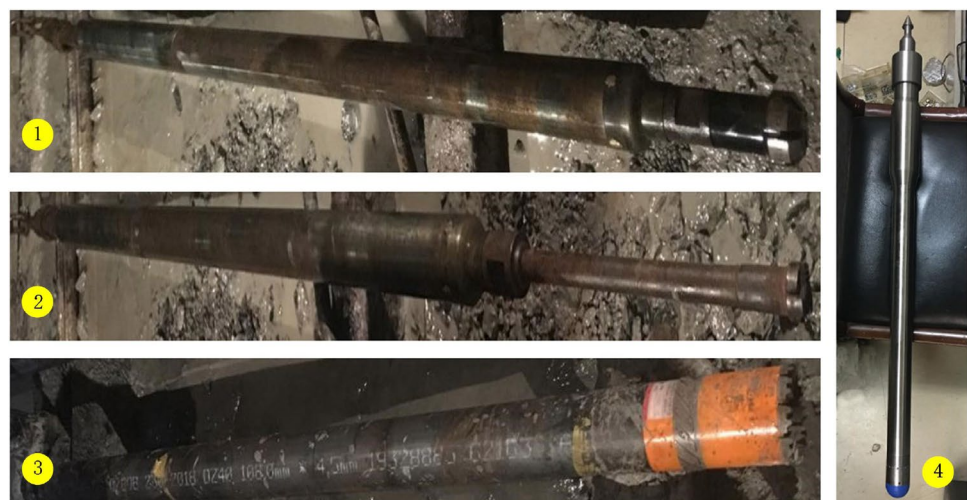
Fig. 9 Auxiliary measurement equipment and diametrical deformation measurement equipment
