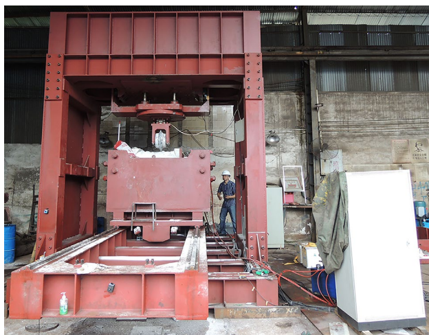
Fig. 16 Linear cutting experimental machine of Beijing University of Technology. (zhao et al. 2015)
