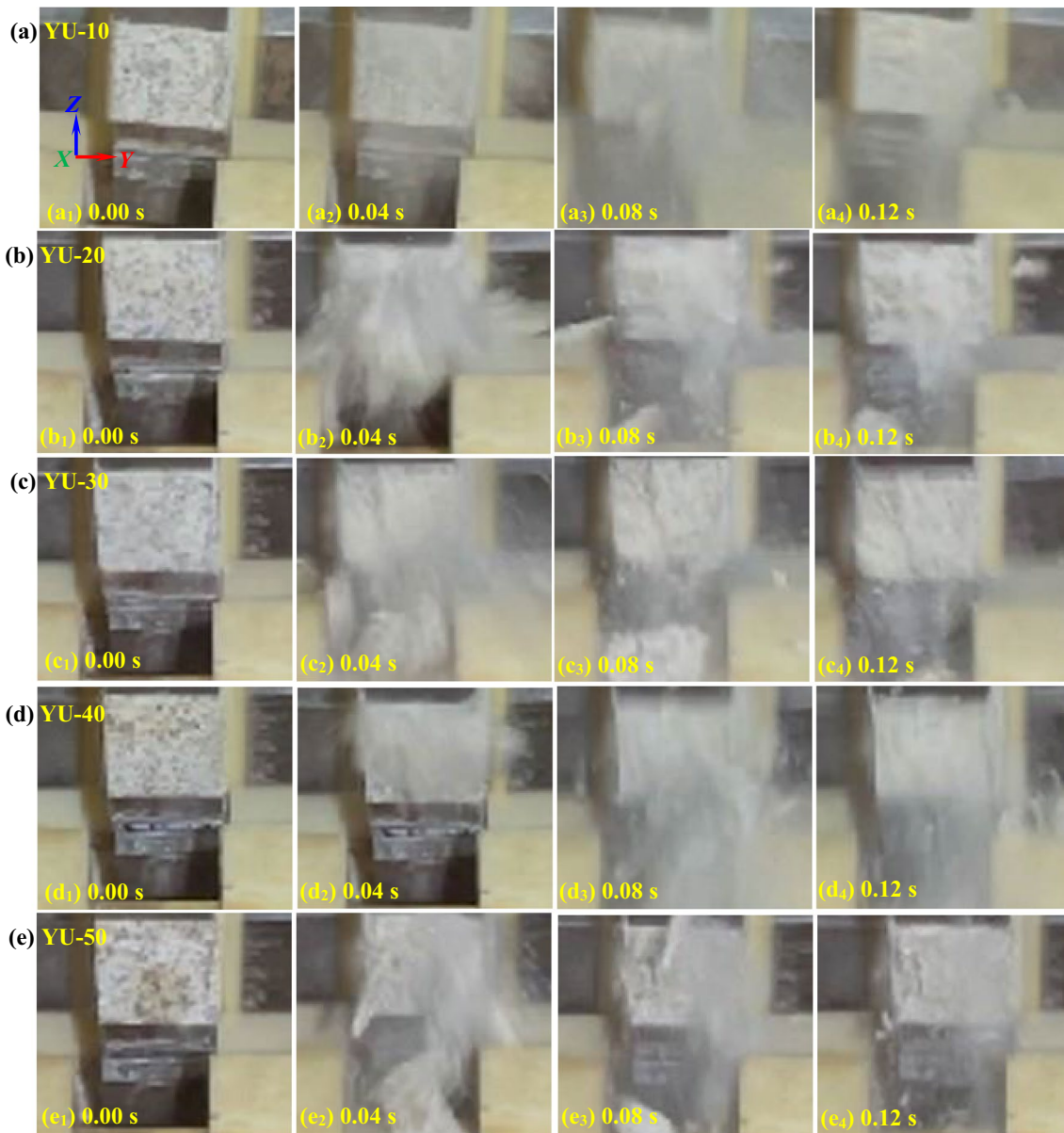
Fig. 8 Rockburst failure process in YU test
