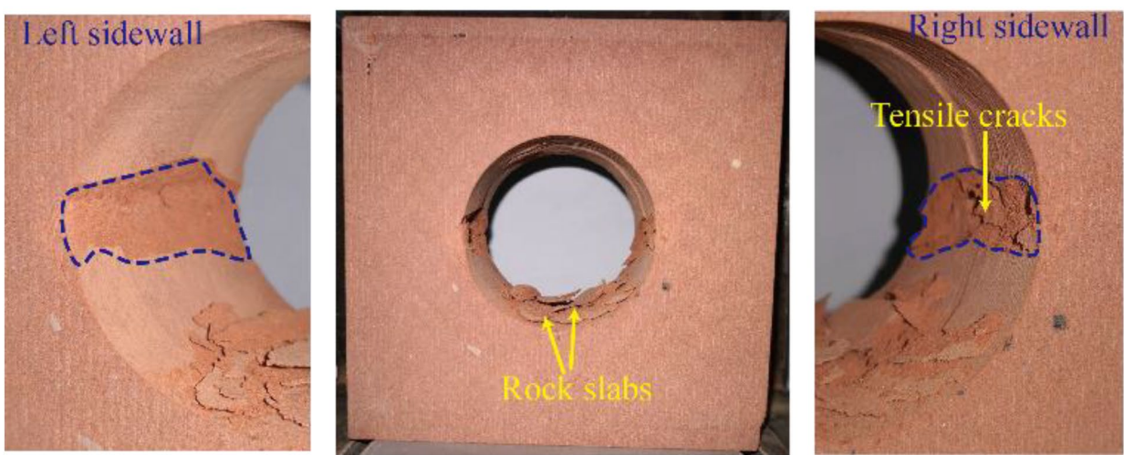
Fig. 21 Photos of specimens after spalling failure
