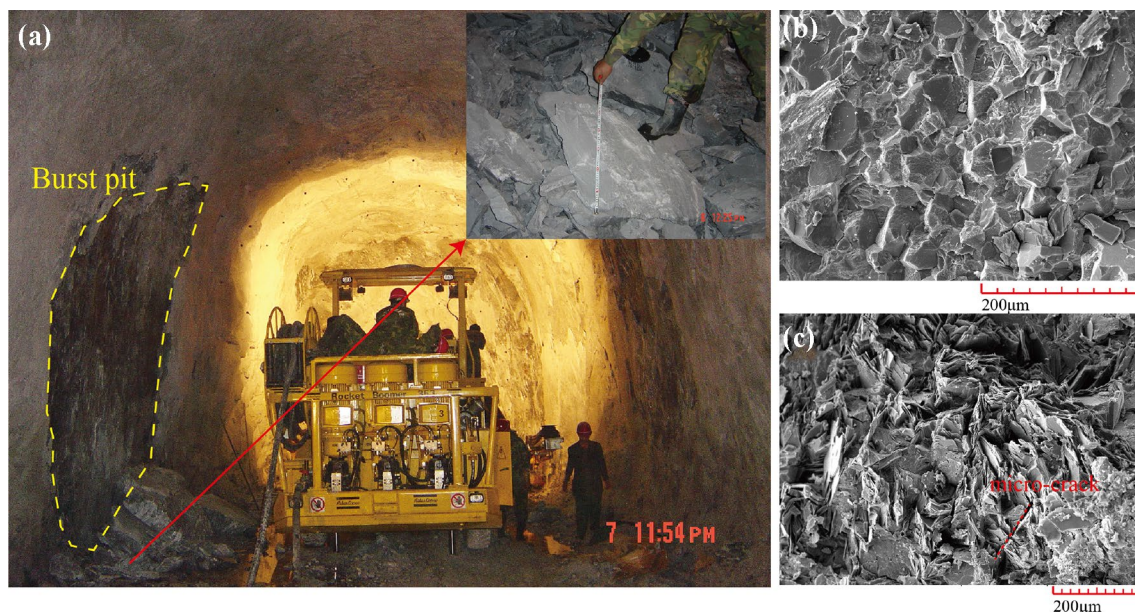
Fig. 1 a Sampling site of the marble samples, b high resolution SEM images of dolomite crystals, and c flaky chlorite
