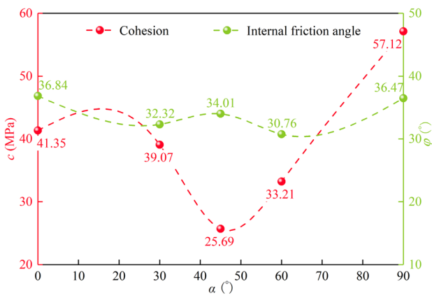
Fig. 14 Variation of cohesion c and internal friction angle \varphi with bedding angle \alpha
