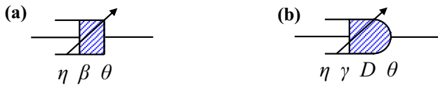
Fig. 7 Fractional components for transversely isotropic rock: a fractional Abel dashpot; b fractional nonlinear damage dashpot
