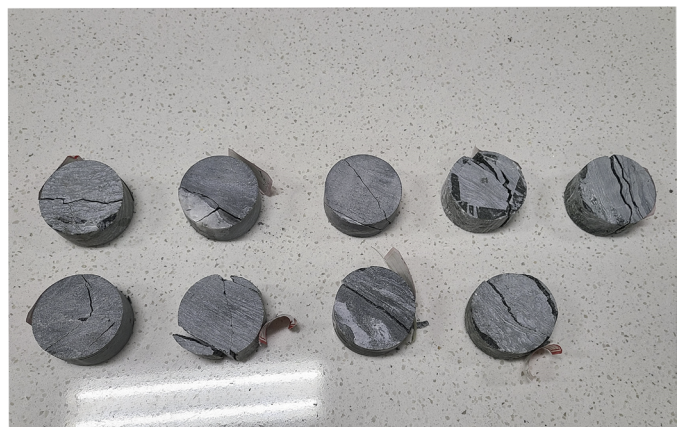
(b) Rock sample after test
