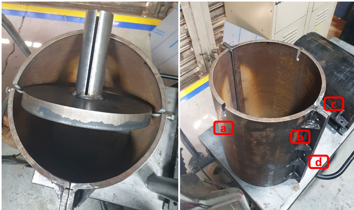
Fig. 3 External confinement: a the slot for base plate wings, b reinforcing gussets, c flanges, and d holes for the bolts
