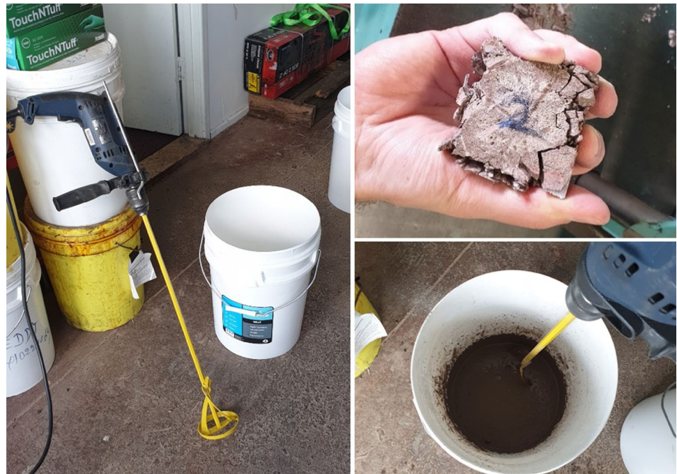
Fig. 9 Grout mixing stages and a 50×50×50 mm sample after the test
