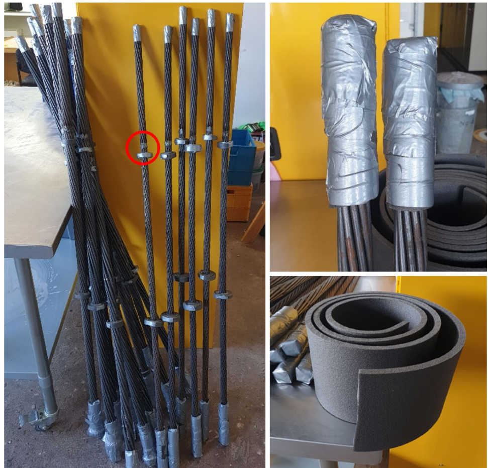
Fig. 8 Process of using closed cell foam to create an ungrouted section and centre the cable during the grouting—the red circle is the centralizer foam
