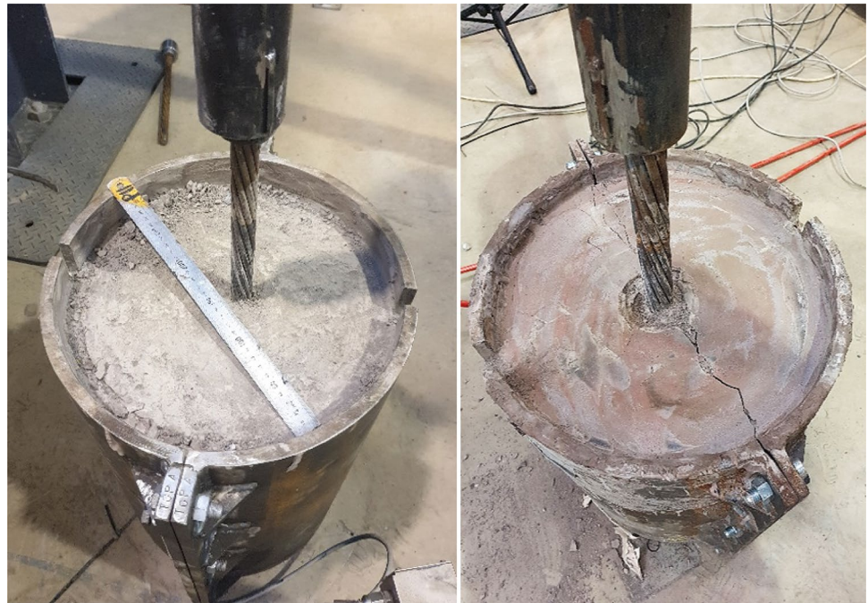
Fig. 20 Left: absence of radial crack in superstrand cable, and right: radial crack in 9 strand cable
