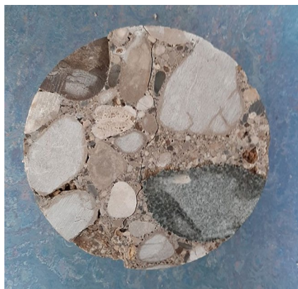
Fig. 2 Typical crack observed after intact specimen failure during uniaxial testing
