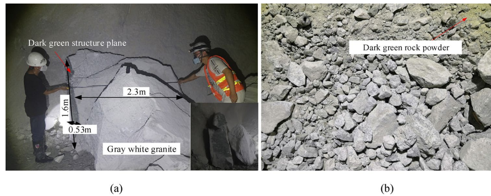
Fig. 4 Shape of rock blocks from the rockburst. a A large rock block with a size of 2.3 m × 1.6 m × 0.53 m, and b rock grains and dark green rock powders
