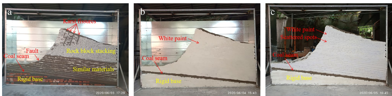
Fig. 6 Model making steps 5 and 6: a model production completed; b apply white paint on the model surface for smooth treatment; c Scattered spots are painted on the model surface randomly
