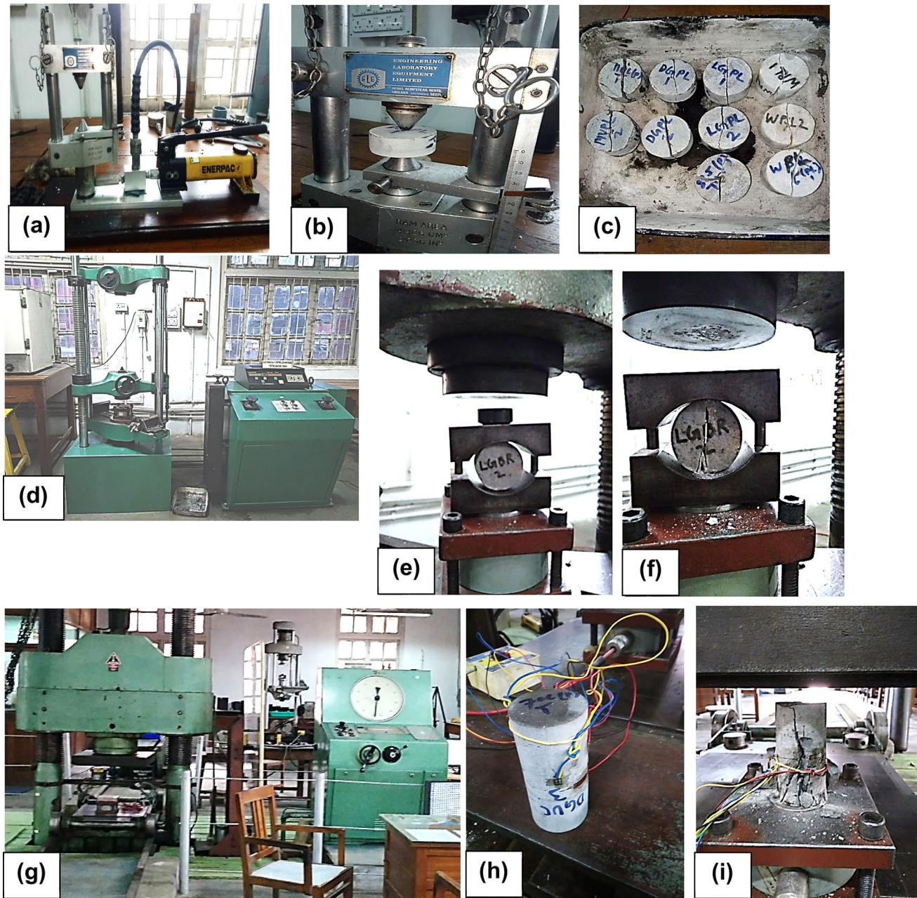
Fig. 8 Laboratory experimental set up for determining engineering geological properties of intact rocks. a–c Point load Strength Index (PLSI); a equipment set up, b specimen under test, c Specimens after first round of PLSI test; d–f Brazilian test; d equipment set up, e specimen for test loaded between platens before testing, f specimen after test; g–i uniaxial compressive strength (UCS); a The Univer-
