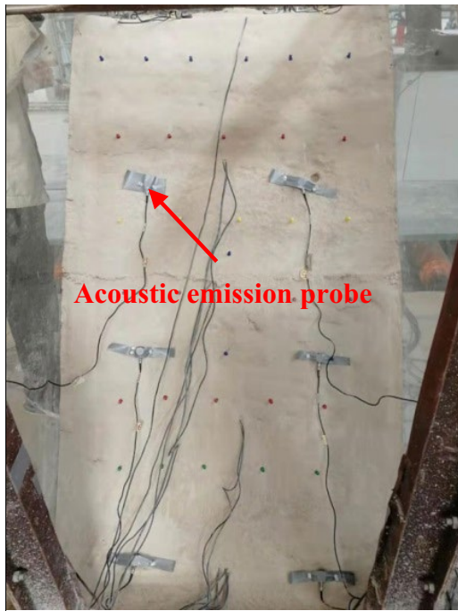
Fig. 5 Layout of acoustic emission probe
