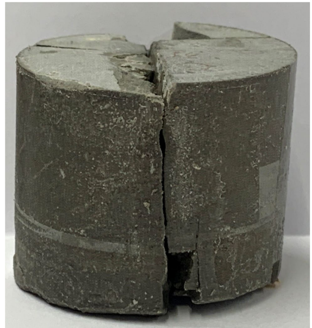
Fig. 2 Picture of a COx sample fractured using the direct shear device
